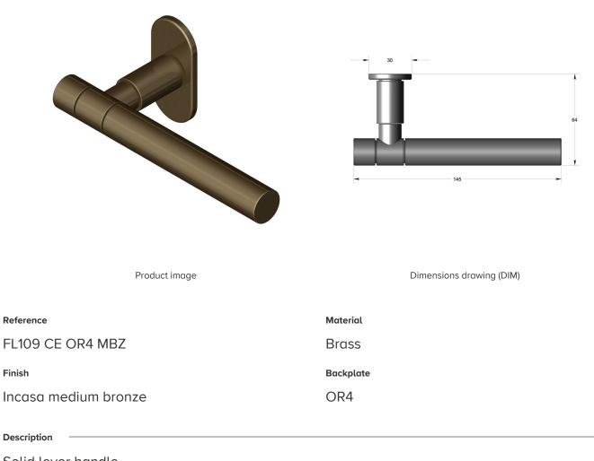
Solid lever handle Concealed fixing High performance bearing rose Back to back fixing Conforms to EN1906 high usage Suitable for us on fire doors
